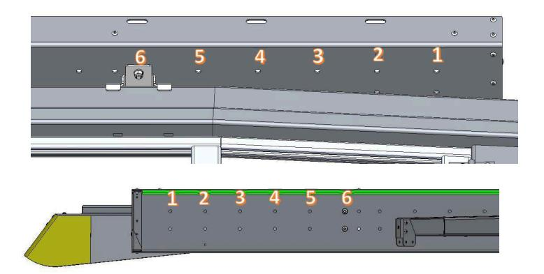
Once you've marked the position of the holes on the base of the, you can proceed to drill the holes into the base as shown below.
