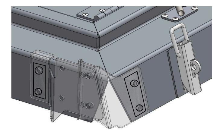
Once all the holes are drilled and the sealant is applied. You can now mount these brackets using the bolts supplied as shown in the drawing provided on page 3.
