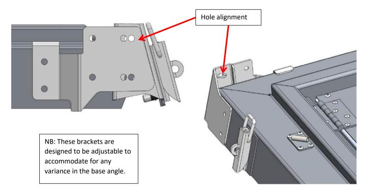
Once the brackets are aligned, you can now mark the area of the base where you would be required to drill your holes.
