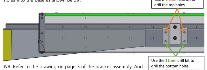
use the same method of applying the sealant on and around the holes of the bracket such as the previous bracket. Once mounted, the awning will align with the Roof Conversion, as shown below (arms, canvas and bag removed for clarity):
