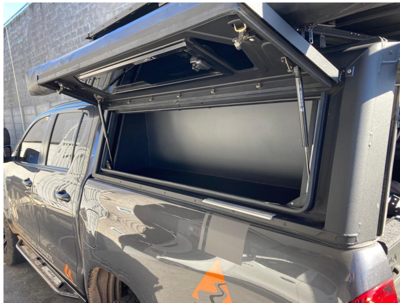
Photo of Canopy cupboard fitted into canopy.
